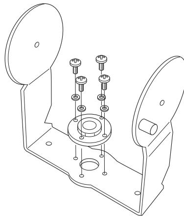
**Figure 5.8** Attaching the plate to the suspension bracket
