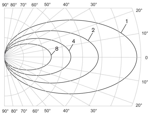
**Figure 4.5** Polar diagram of the radiation pattern for 1, 2, 4 and 8 carriers
