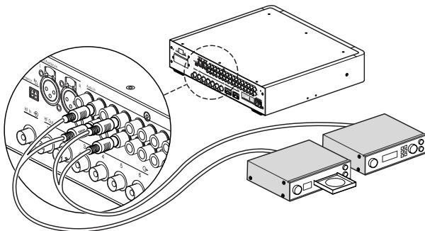
**Figure 6.3** Connecting external audio sources to the Modular IR transmitter
