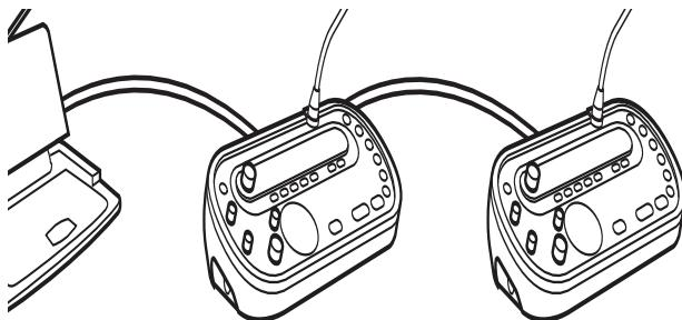
**Figure 6.1** Connecting the optical network to the modular IR transmitter
