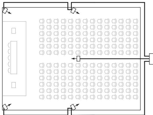
**Figure 4.24** Symmetrical arrangement of radiator cabling (recommended)
