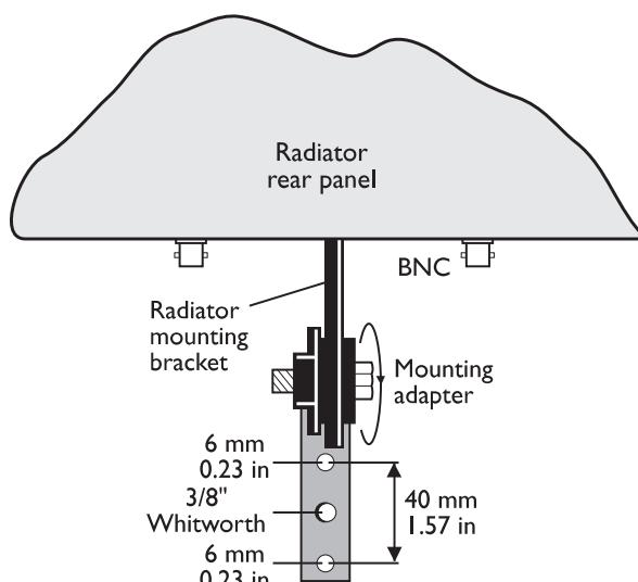
Figure 5.15 LBB 3410/05 Radiator Mounting
