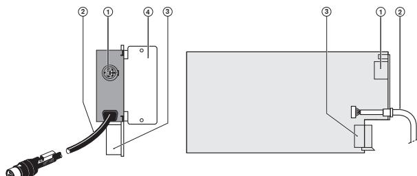
**Figure 3.4** Integrus DCN interface module
