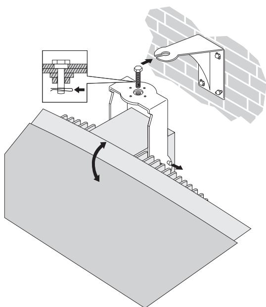
**Figure 5.14** Attaching the radiator to the wall mounting bracket
