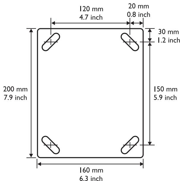
**Figure 5.13** LBB 3414/00 wall mounting bracket showing dimensions and drilling pattern
