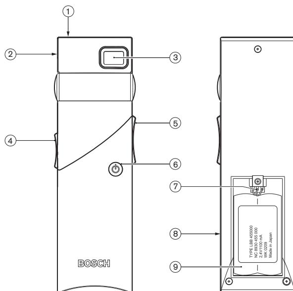
**Figure 3.10** Receiver, front view and back view with open battery compartment
