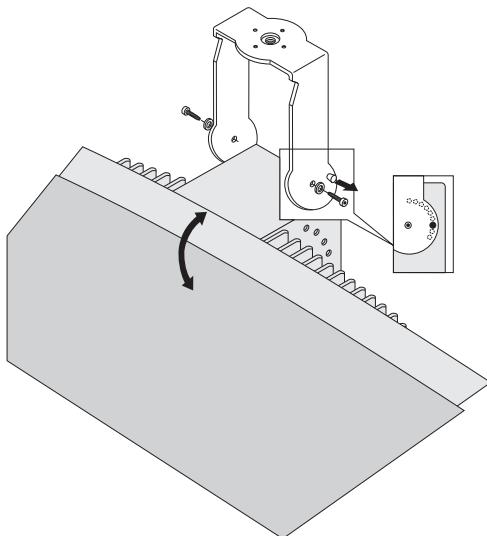
**Figure 5.9** Attaching the suspension bracket to the radiator
