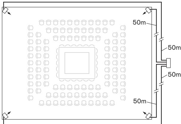
**Figure 4.22** Radiators with equal cable length
