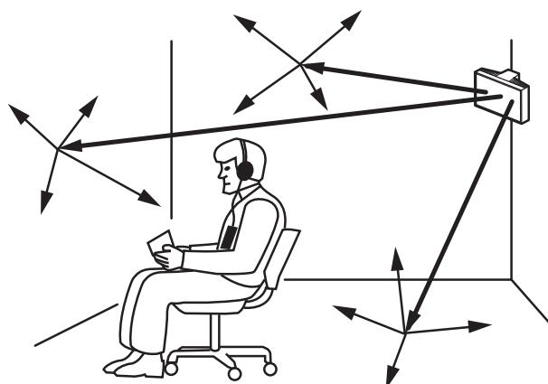
**Figure 4.13** Combination of several reflected signals
