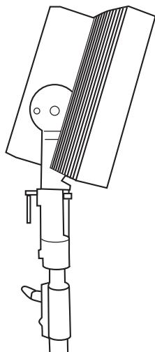
**Figure 5.11** Attaching the radiator inclusive suspension bracket and stud to the floor stand
