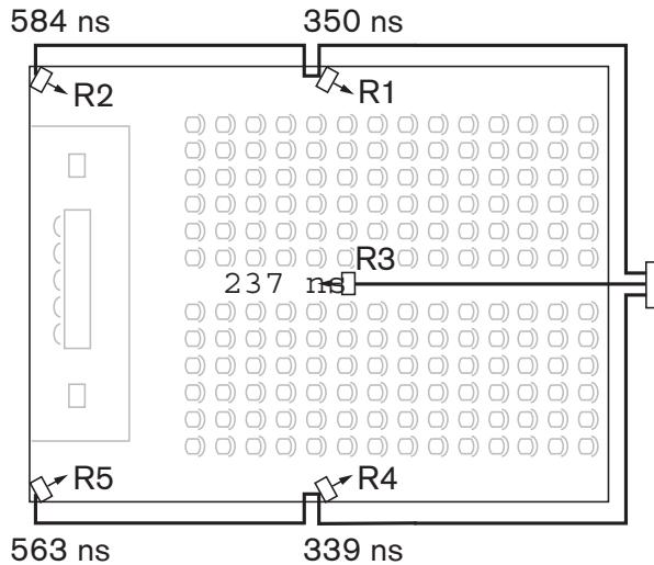
**Figure 7.4** System with five radiators and measured impulse response times
