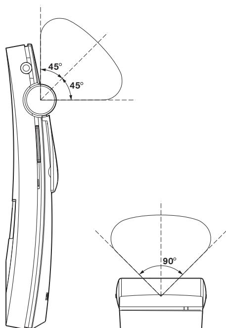
**Figure 4.3** Directional characteristics of the receivers
