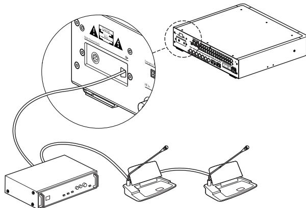
**Figure 6.2** Connecting the DCN systems to the Modular IR transmitter
