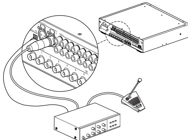
**Figure 6.4** Connecting an emergency signal
