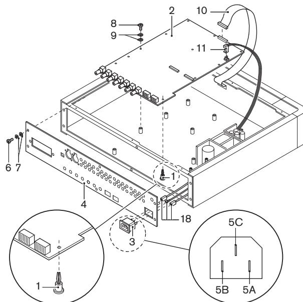
**Figure 5.6** Installation of the INT-TXK (steps 1 - 6)
