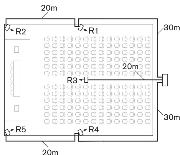
**Figure 7.3** System with five radiators and measured cable lengths
