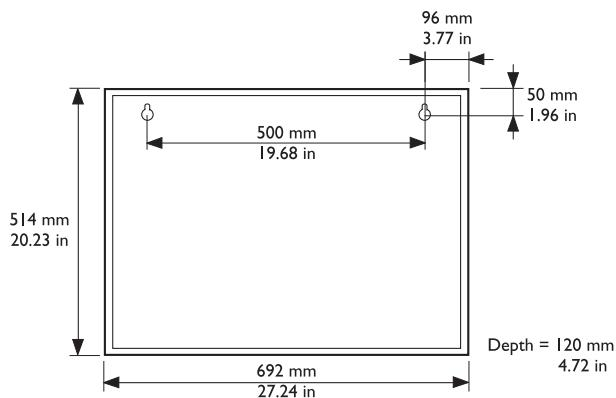
**Figure 5.16** Charging cabinet mounting dimensions
