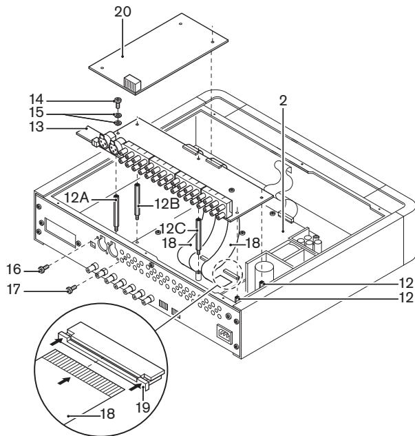
**Figure 5.7** Installation of the INT-TXK (steps 7 - 12)
