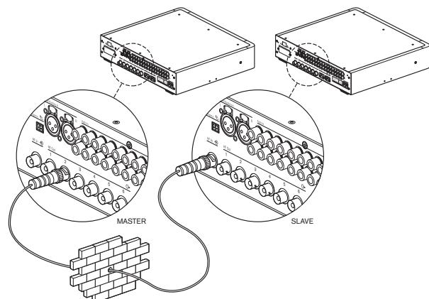
**Figure 6.5** Connecting to another transmitter
