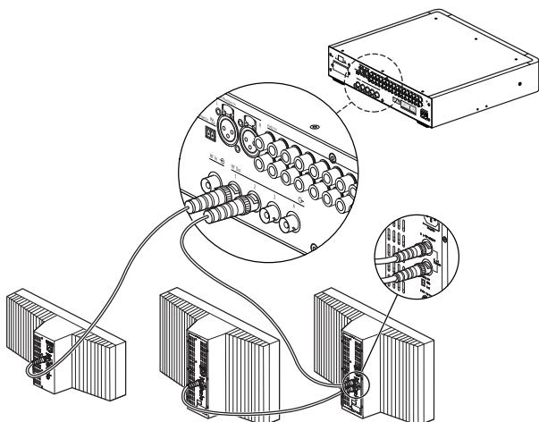
**Figure 6.6** Loop-through connection of radiators
