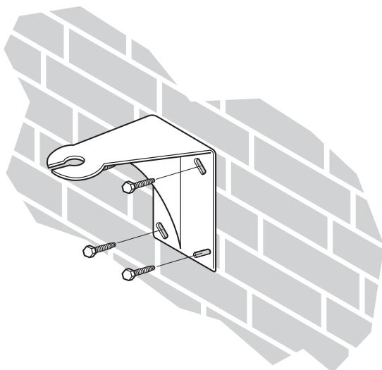
**Figure 5.12** Attaching the wall mounting bracket to a wall
