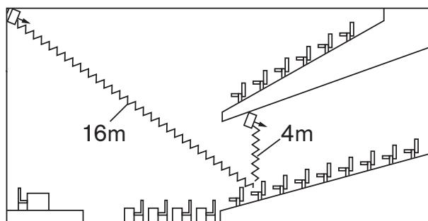
**Figure 7.6** Radiation path length difference for two radiators
