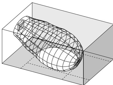
**Figure 4.6** The radiator mounted at 15° to the ceiling
