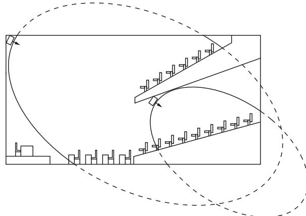
**Figure 4.16** Radiator for covering seats beneath a balcony
