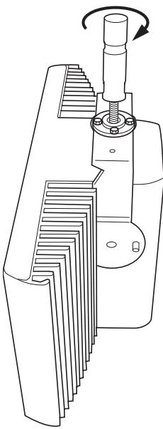
**Figure 5.10** Attaching the stud of a floor stand to the suspension bracket of the radiator
