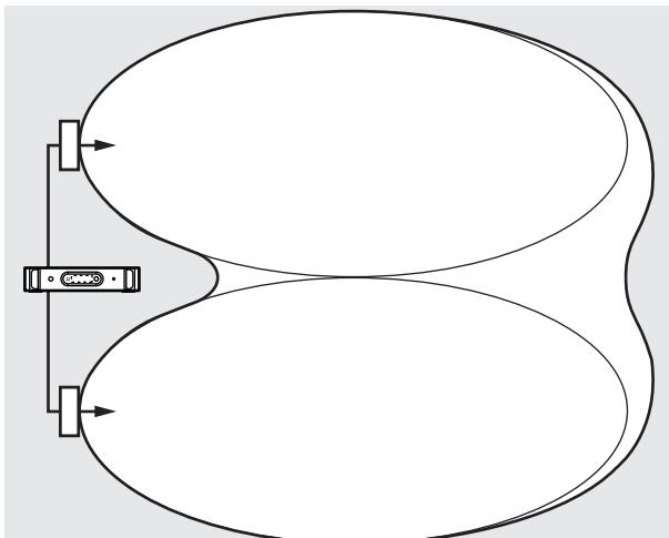
**Figure 4.17** Increased coverage area caused by added radiation power
