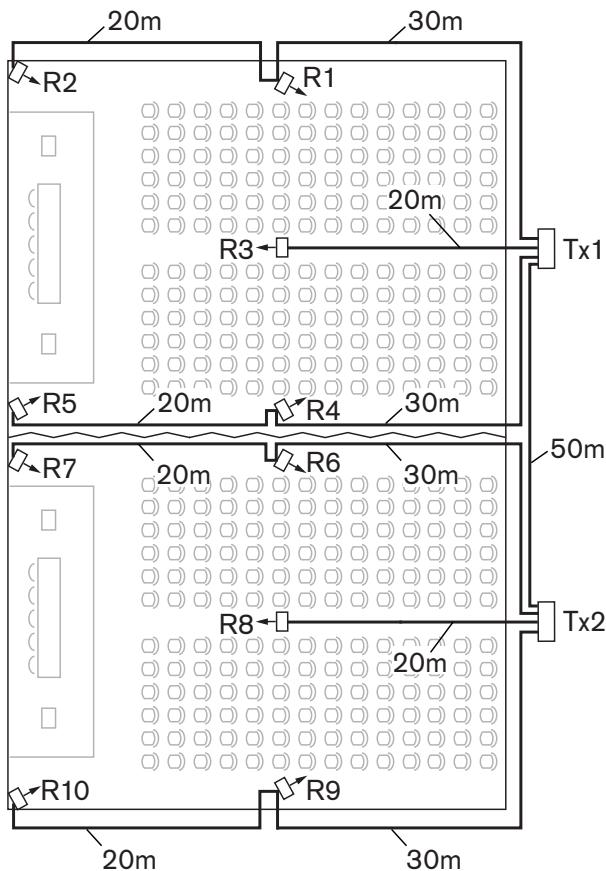
**Figure 7.5** System with master and slave transmitter in multi purpose room
