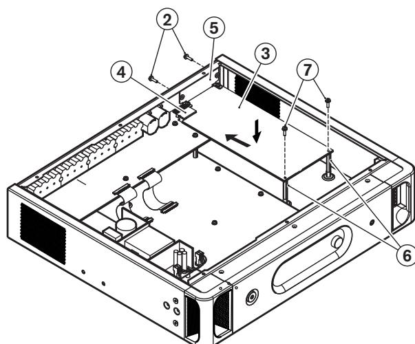
**Figure 5.3** Mounting an interface module in the transmitter housing
