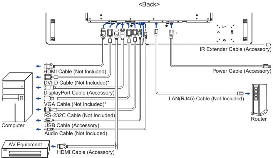
\* Cable is not supplied with the monitor. If you use low quality Cable, it may cause a result of electro-magnetic interference. Please contact the iiyama Support Centre in your country if you wish to connect the monitor via the VGA or DVI input.
