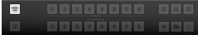
Press and release the **Control Lock** button to toggle between the control lock states.
