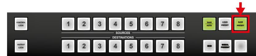
Step 2. Press and release the desired **source (memory address) button** (source 1 to 8). Now the current configuration is stored in the selected memory.
