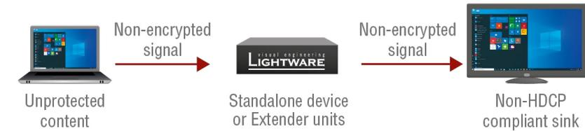
Setting the HDCP parameter to Auto on the output port and disabling HDCP on the input port, the transmitted signal will not be encrypted if the content is not protected. Thus, non-HDCP compliant sinks will display non-encrypted signal.
