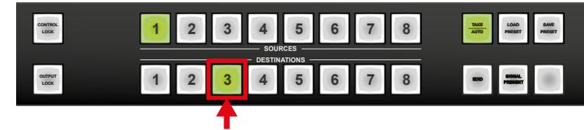
Now the source button that is connected to the selected destination will light up. If no source button shines, the selected destination is in muted state. Upon pressing another destination button, the last state of the destination can be seen.
