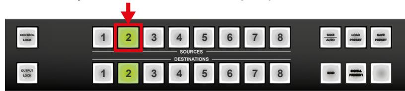
**Step 2.** Press and release the desired **destination buttons** that need to be (dis)connected to/from the selected source. The preselected destination buttons will blink.
