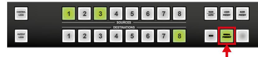
**Step 2.** Input buttons will light up indicating that active TMDS clock signal is present on the respective input connectors. Output buttons will also light up indicating that a powered monitor is attached to the output. The output circuit senses TMDS pull-up resistors on the monitor side.
