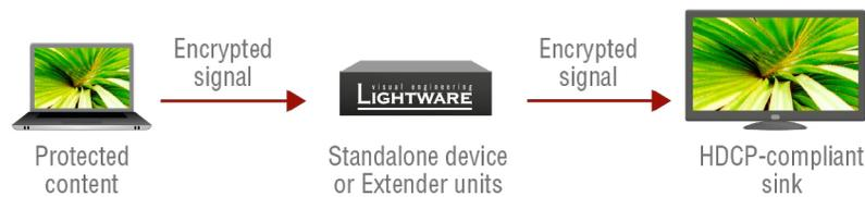
All the devices are HDCP-compliant, no manual setting is required, both protected and unprotected content is transmitted and displayed on the sink.
