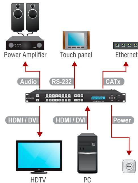
**HDMI / DVI** Connect an HDMI/DVI cable(s) between the source(s) to the input port(s) of the matrix.
