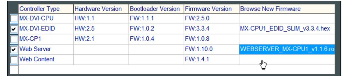
Load the new firmware files for each controller; click on the cell in the Browse New Firmware column of the desired controller (see the pointer on the picture above). A dialog window pops up to confirm whether you really want to load a new firmware (modify the path). Now you can browse the new firmware file. After opening the new file, the cell will contain the name of the firmware file.
