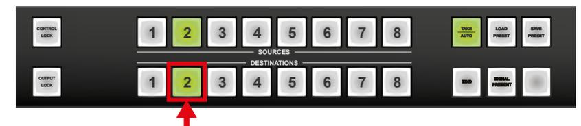
**Step 2.** Press and release the **Output Lock** button; it lights up in red, and lock function is activated at once. No source can be changed at the locked destination.
