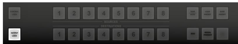
Destinations can independently be locked or unlocked. Locking a destination does not affect other destinations.
