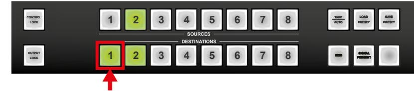
**Step 3.** Press and release **Take** button; the selected input is switched to the selected output(s).
