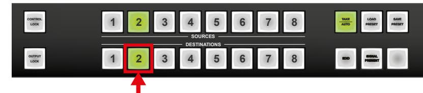
**Step 2.** Press and release the desired source button. The switch action will be executed immediately. Switching between sources to the selected destination can be done directly.
