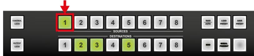
The sample drawing shows that Input 1 is currently connected to the Output 2, 3, and 5 ports.
