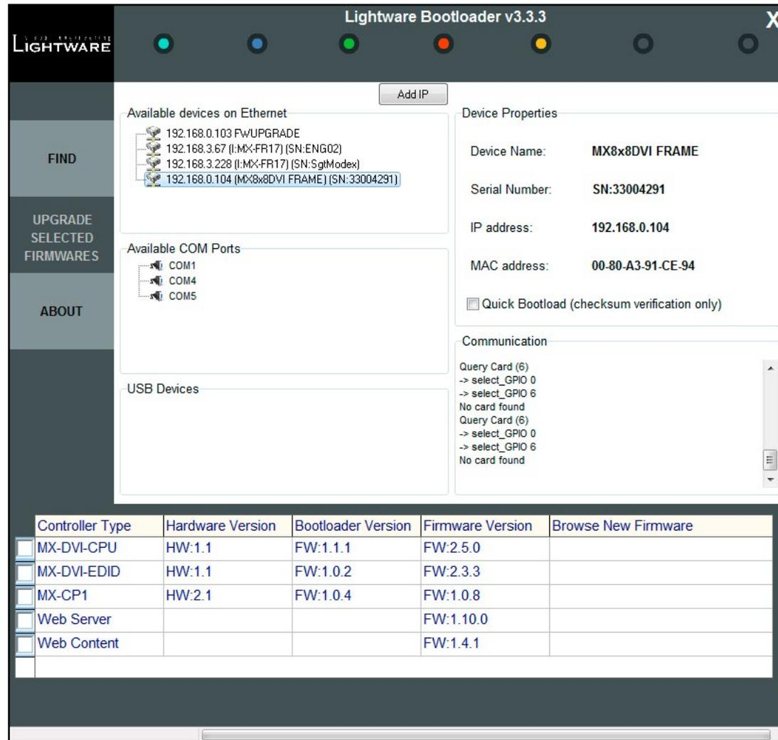
**Lightware Bootloader – Details of the Device**
