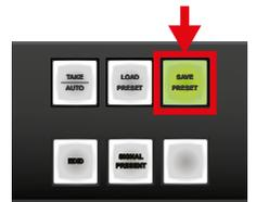
**Step 5.** A light sequence will occur to confirm the command. (Take/Auto, Load Preset and Save Preset buttons will light up one after the other)
